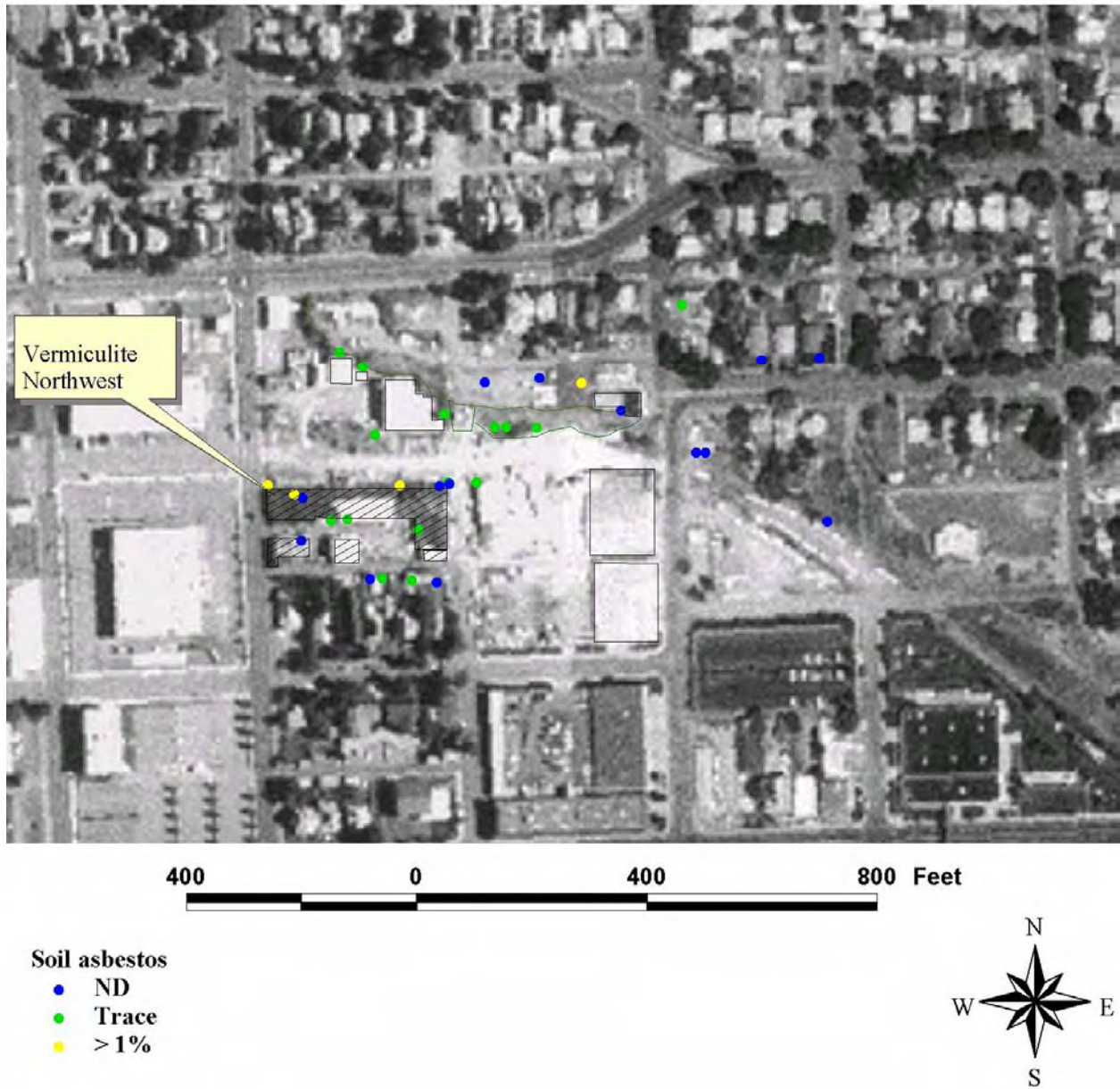
Figure 4 - Soil Sample Locations near Vermiculite NW site. Spokane, WA. 16,17
