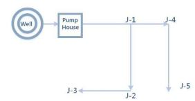
Pump lift from water level in the well to the top of the well casing = 119.3 ft
