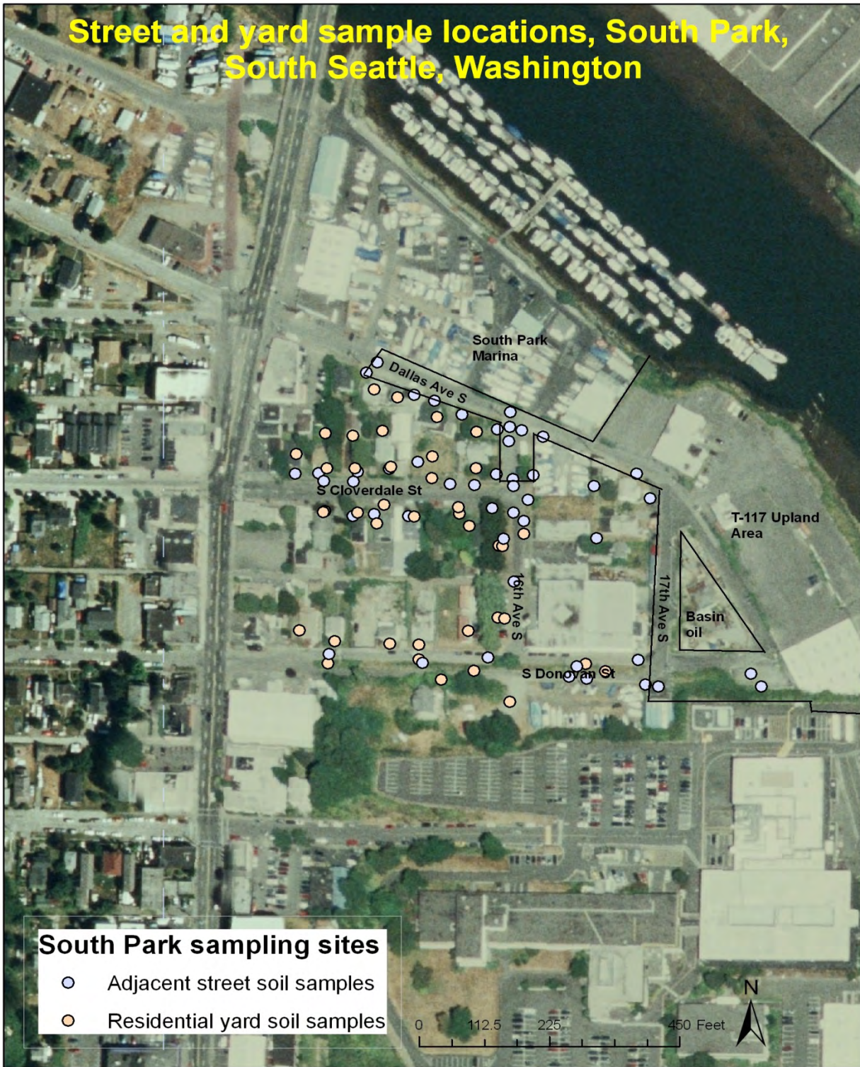
Figure 2: Soil sample types and locations at South Park site, 2008 and 2009, South Seattle, King County, Washington.
