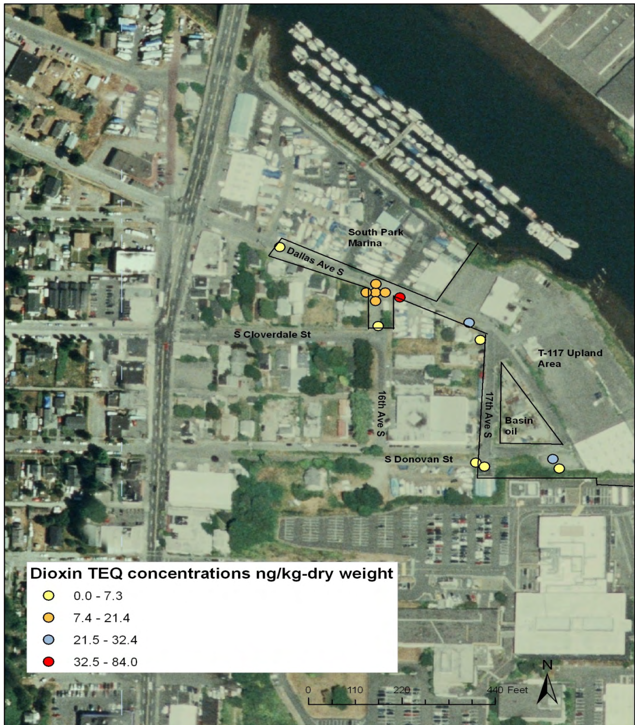
Figure 5. Dioxin TEQ concentrations in dry weight (ng/kg) in surface soil (0.1 – 1 feet) at the streets, South Park site, 2008, Seattle, King County, Washington.
