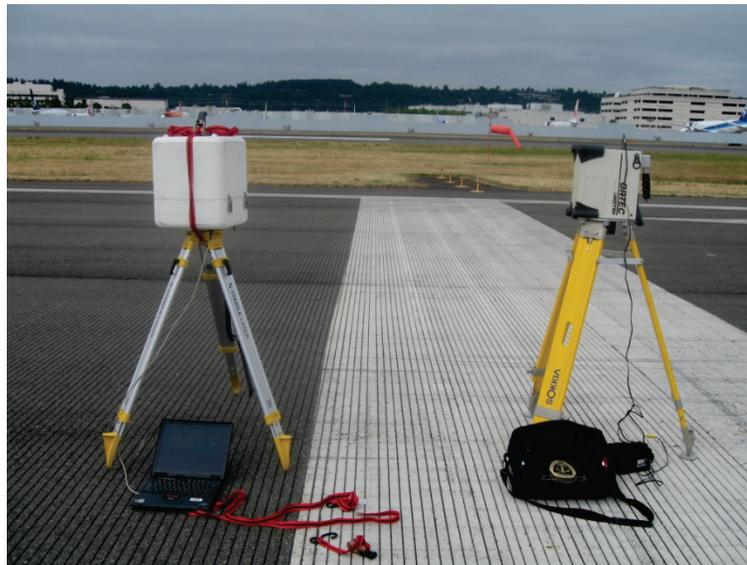
Figure 14. The PIC (left) and HPGe (right) used for measurements at the land test line.
