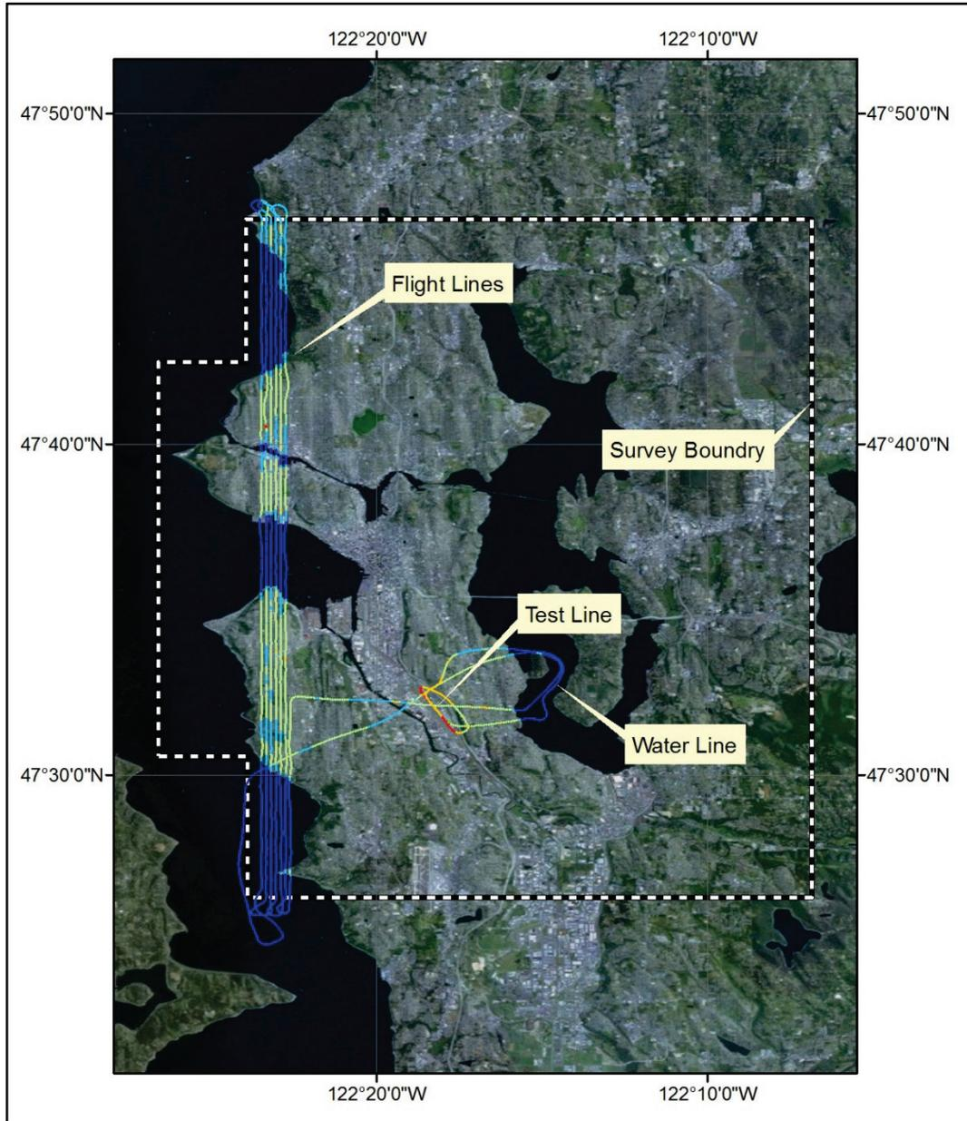
**Figure 19. Survey flight components.**
