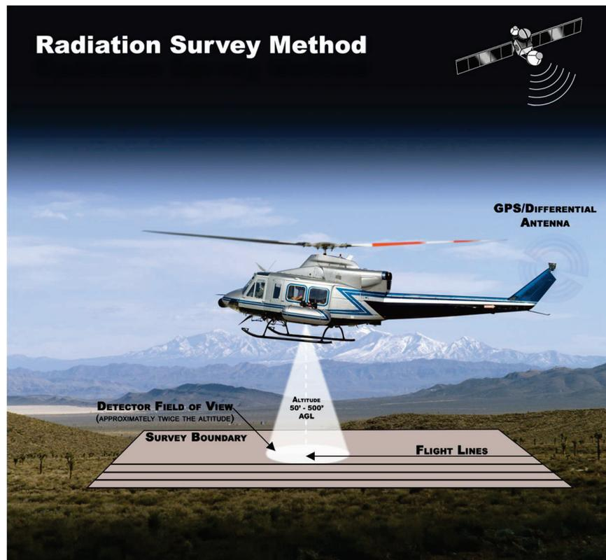
**Figure 5. Methodology of the aerial radiation survey.**
