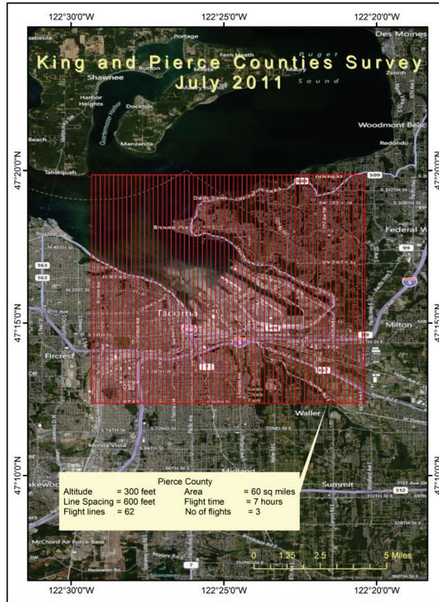
**Figure 2. Pierce County survey area and planned flight lines.**
