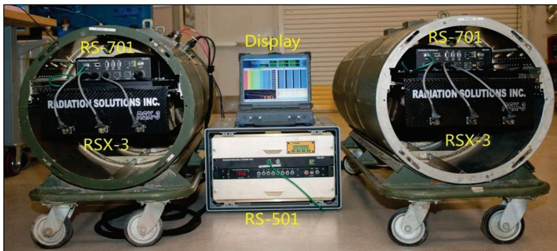
**Figure 8. Components of the AMS RSI Aerial Radiation Data Acquisition System.**
