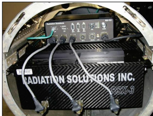
**Figure 10.** *The RS-701 console on top of the RSX-3 detector box.*
