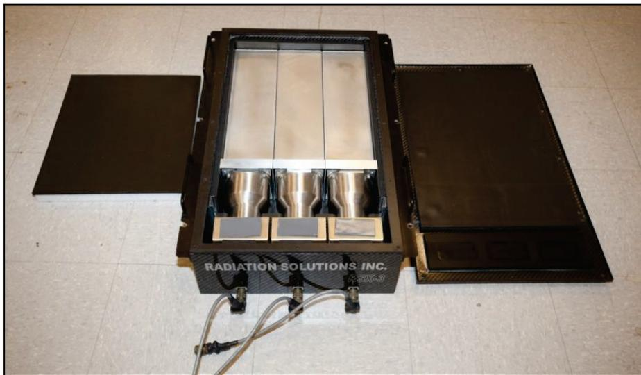
**Figure 9. RSX-3 box with three 2"×4"×16" sodium iodide thallium-activated Na(Tl) crystals, three PMTs, and ADS modules.**
