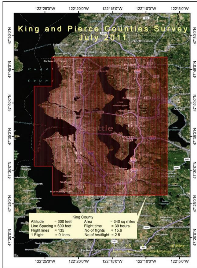
**Figure 1. King County survey area and planned flight lines.**
