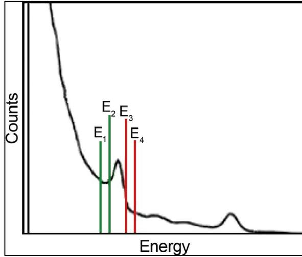
Figure 15. 3-window algorithm applied to a typical spectrum.
