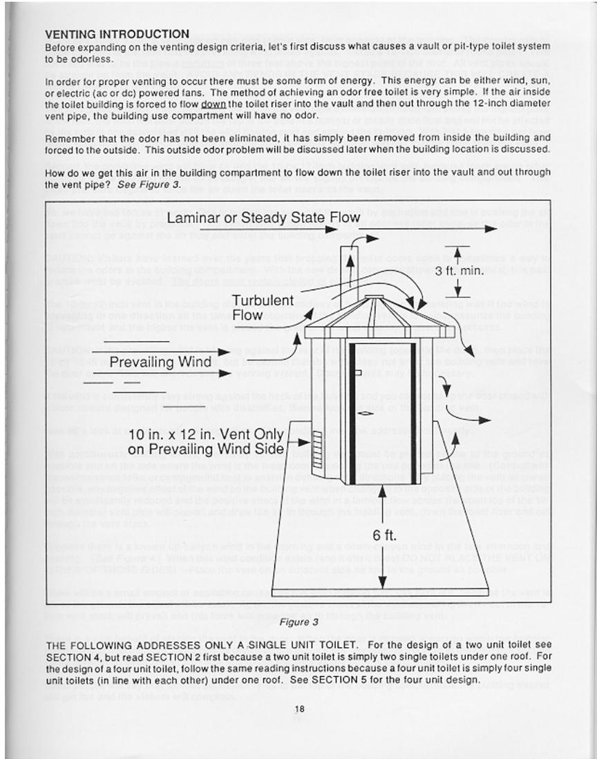
**Figure 2. Vault Toilet with Passive Ventilation**
