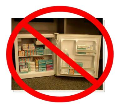
Dormitory-style (or bar-style) units pose a significant risk of freezing vaccine even when used for temporary storage.
