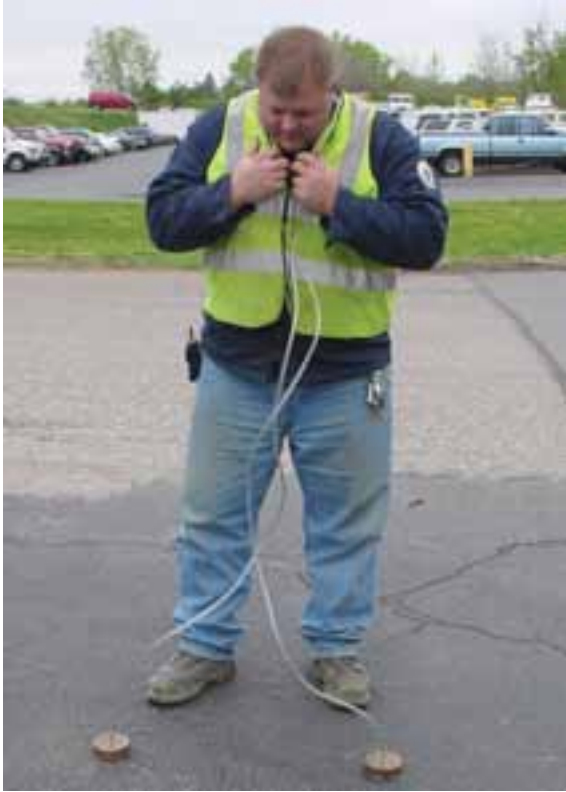
Left: Luther Bitzel of the Columbus Ohio Distribution Group shows the correct way to use Geophones® when working above a water line.
