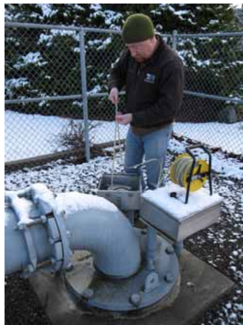
Todd Shepherd, water quality specialist for Tacoma Water, uses an electric water level probe to measure the water level in Well 6B.
