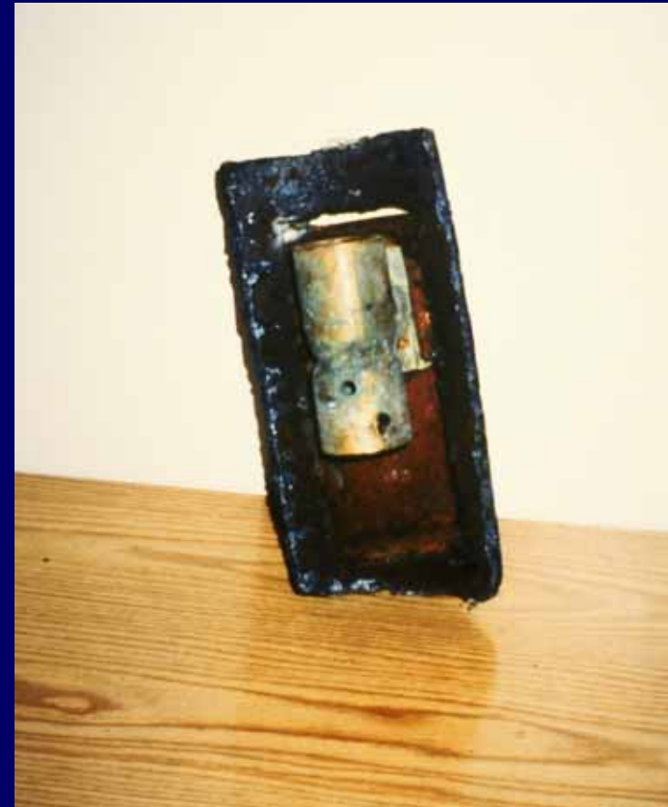
Improperly installed Pitless Adaptor.
