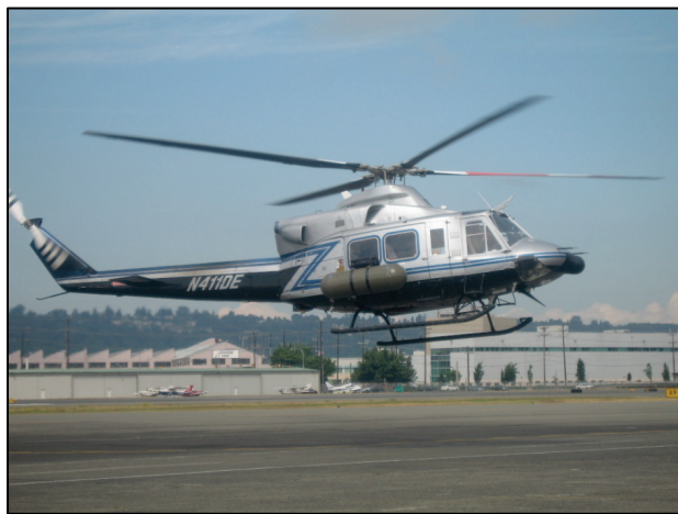
Figure 3. AMS Bell 412 helicopter with externally mounted radiation detector pods.
