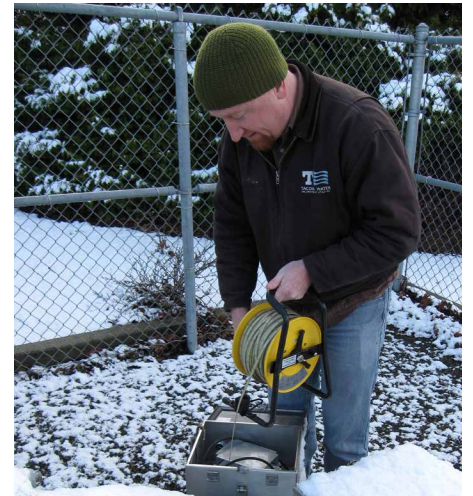
In 2009, Todd Shepherd, water quality specialist for Tacoma Water, uses an electric water level probe to measure the water level in Well 6B. Photo courtesy of Tacoma Water.
