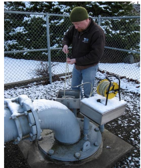
Todd Shepherd, water quality specialist for Tacoma Water, uses an electric water level probe to measure the water level in Well 6B. (Photo courtesy of Tacoma Water.)
