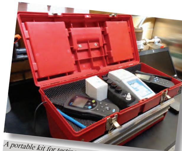
*A portable kit for testing on-line monitoring equipment.*
