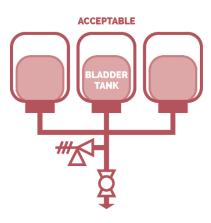
tank. The PRV will protect the tank from excessive pressure that could be generated by an air compressor used to charge the tank.
